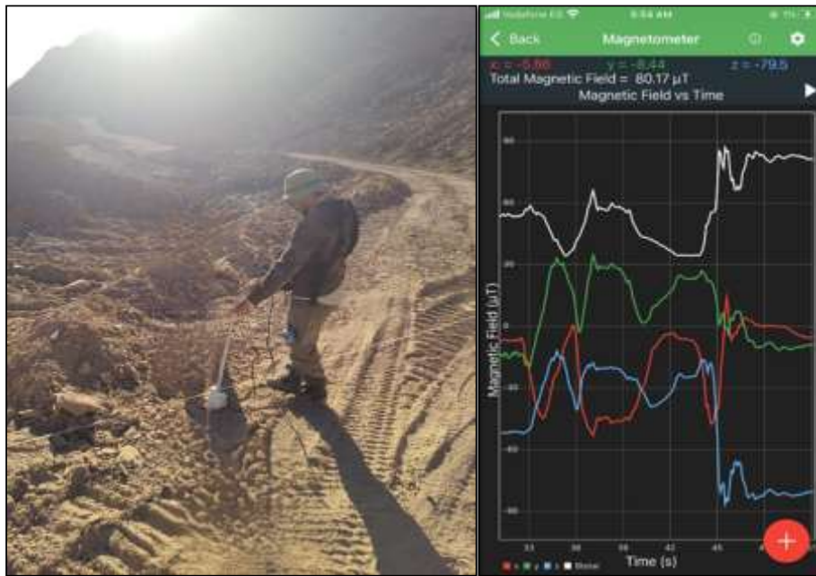
Figure 4: Magnetic data acquisition using magnetometer and smartphone application.
