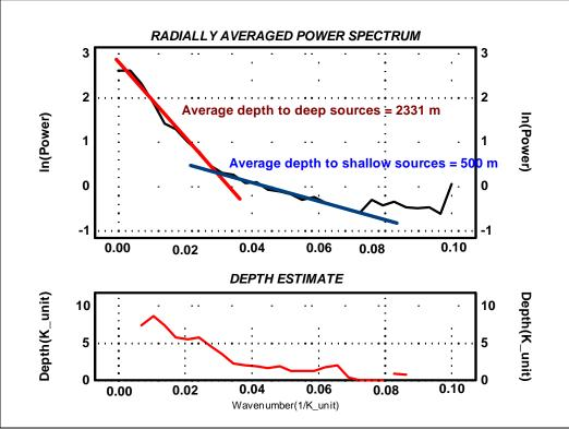
Figure 6: Radially Averaged Power Spectrum of the RTP magnetic data.
