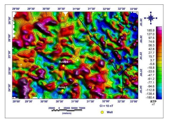
Figure 3: Reduced to the pole (RTP) magnetic map of the study area.
