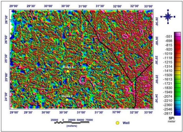
Figure7: Basement depth from Source Parameter Imaging (SPI) technique.
