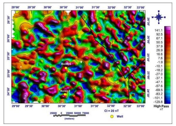
Figure 5: Butterworth High Pass filtered (Residual) magnetic map.
